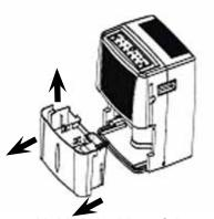
2. Hold both sides of the bucket with even strength, and pull it all the way out from the unit.
